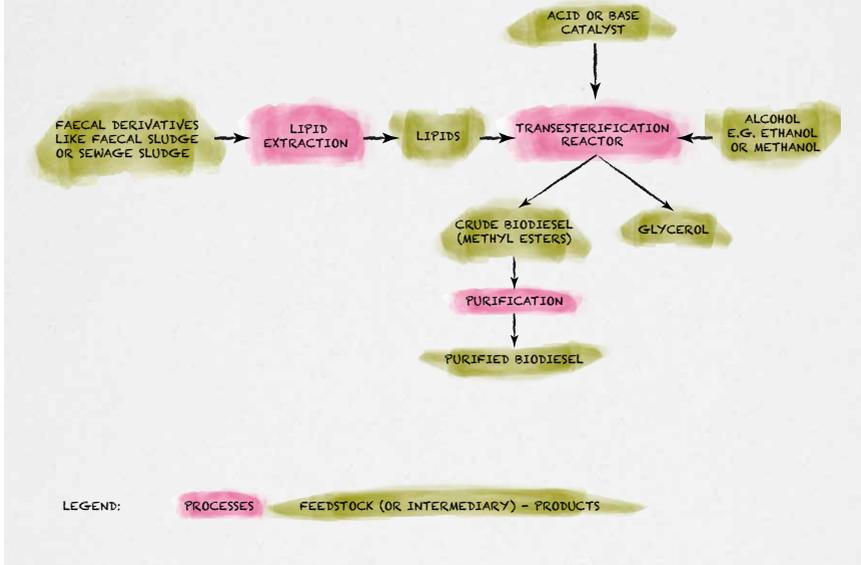
▲ *Figure 3:* Overview of the process and intermediary products from transesterification to produce biodiesel.
