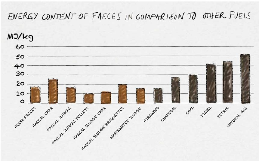
▲ *Figure 1:* The energy content in various forms of faeces in comparison with some common solid and fluid fuels. One MJ (megajoule) equals 0.278 kWh (kilowatt-hours).
