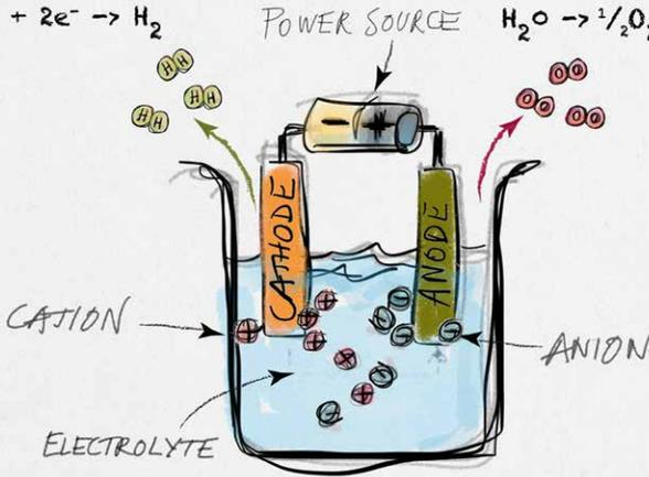
▲ *Figure 2:* Schematic view of an electrolysis cell.
