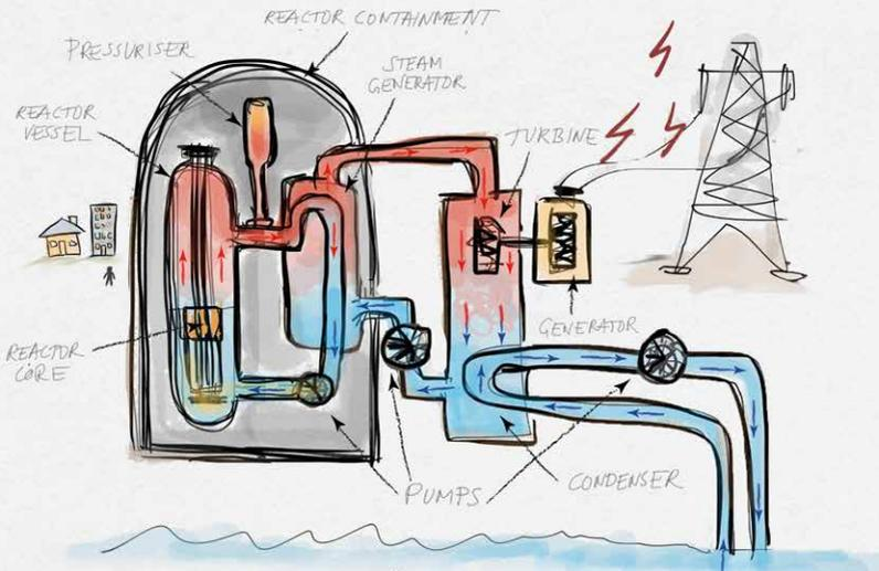
TO PROTECT THE REACTOR FROM OVERHEATING IN CASE OF A BLACKOUT OR IF THE PUMPS SHOULD STOP WORKING, A COMPLICATED AND EXPENSIVE EXTRA COOLING SYSTEM IS REQUIRED.
