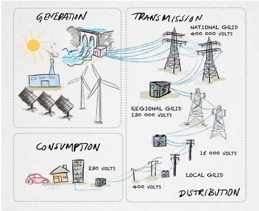
▲ *Figure 1:* Schematic image of the electricity grid.
