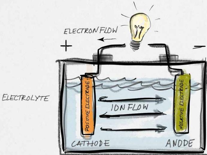
▲ *Figure 4:* Electric current from chemical reactions.
