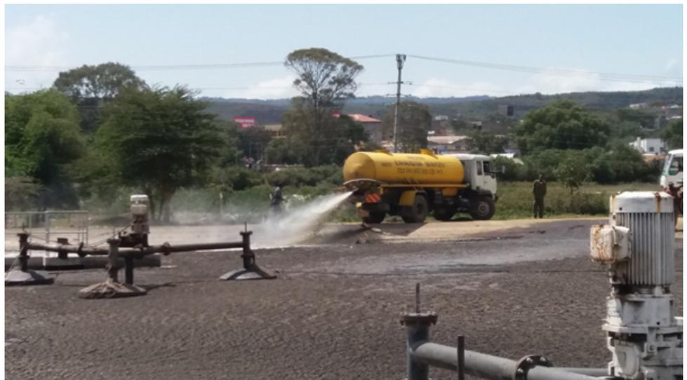
A vacuum truck discharges faecal sludge at the NAIVAWASCO wastewater treatment plant. © DANIEL DDIBA
