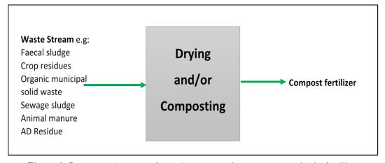
Figure 9: Inputs and outputs from the composting process to obtain fertilizer
