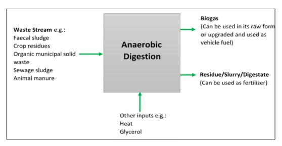
Figure 8: Inputs and outputs from the anaerobic digestion process
