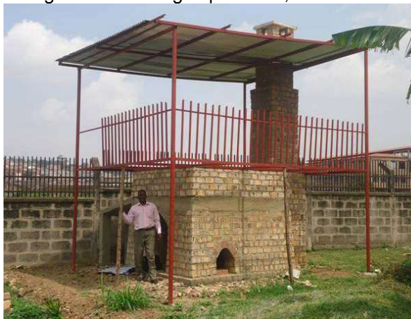
Figure 1: The pilot kiln where bricks were fired using dried FS.
